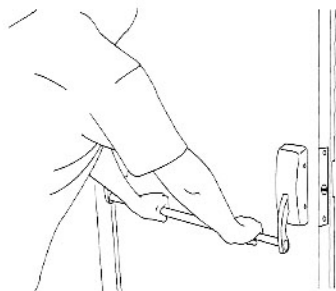
A vertical crossbar on a door affords the user to open the door by pushing.
